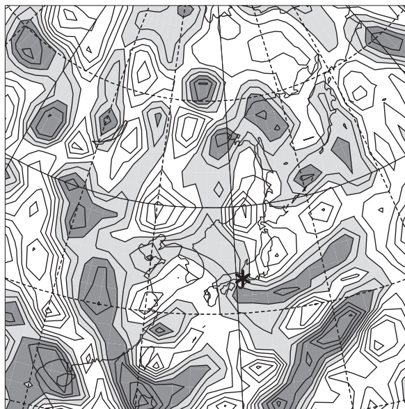
Fig. 5. Horizontal divergence on 10 hPa at 1500 LST 11 May 2006. Contour intervals are 2.5 \times 10^{-6} \text{ s}^{-1} . Negative regions are shaded. An asterisk (*) denotes the observation site.
