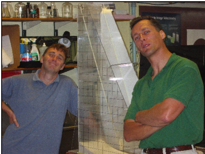
Granular slumping in the lab: Neil Balmforth and Rich Kerswell performing dam-break experiments with granular material. (A gate, suddenly drawn back, releases a pile of grit that cascades down and sweeps to the right in a sliding granular current. The mass eventually comes to rest leaving a slumped deposit.) Picture courtesy of Glenn Jerley.
